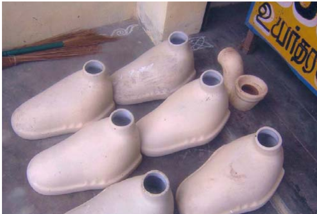
Photo: 34 A Close View of Sanitary Pans & Bent in the RSM in Vellore District
